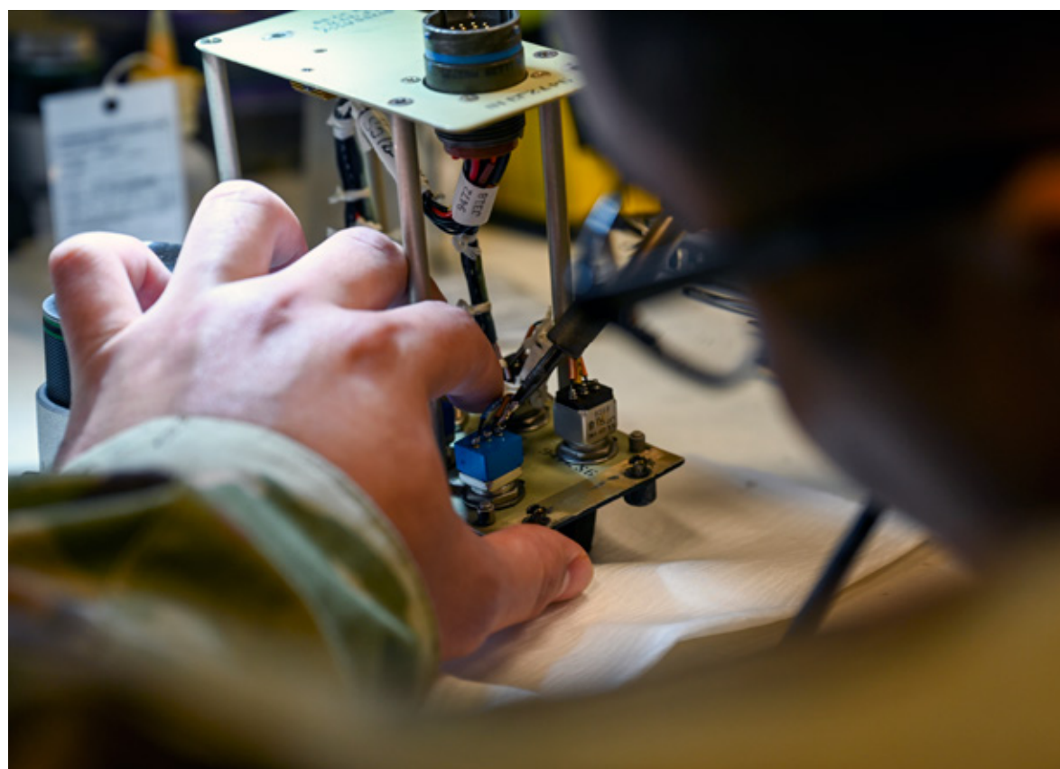
Senior Airman Michael Philip Flores-Rodríguez, 8th Maintenance Squadron AFREP technician, uses a solder to join metals on a fault function panel at Kunsan Air Base, Republic of Korea, May 25, 2025. The strategic approach within the AFREP program allows for maintainers to repair rather than replace equipment, a valuable resource that keeps essential components readily available without relying on external repair locations. ▲
