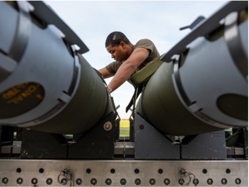
An Airman assigned to the 393rd Bomber Generation Squadron prepares GBU-38 Joint Direct Attack Munitions to be loaded onto a B-2 Spirit stealth bomber at Whiteman Air Force Base, Mo. The loading operations were a component of the Air Force Research Laboratory QUICKSINK Joint Capability Technology Demonstration, a new low-cost, air-delivered capability for defeating maritime threats. (U.S. Air Force photo by Senior Airman Joshua Hastings) ▲
